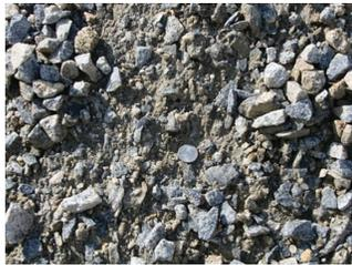
Aggregate is used to make roads. It is mostly limestone with sand mixed into it.
