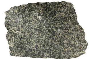
Diabase is an igneous rock believed to have formed from cooling lava. It is mined for use in construction. The miners of Chester County called it "black granite."
