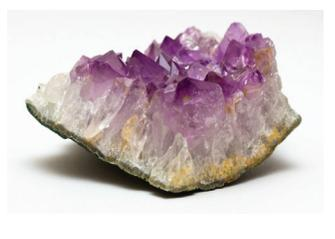
Amethyst is a type of quartz,  $\text{SiO}_2$ . The color comes from small amounts of iron and from radiation during formation.
