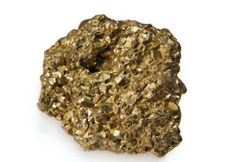
Pyrite is known as "fools gold" and has little commercial value. It is made of iron and sulfur.
