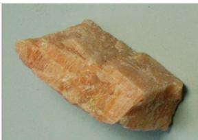
Feldspar is one of the mineral building blocks of igneous rocks like granite. Tiny fragments of feldspar can be seen in sand.
