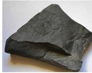
Shale is one of PA's most abundant rocks. It is made of ancient mud that turned to rock.
