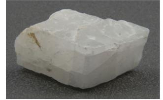
Calcite is made of calcium, carbon and oxygen. It is a major component of limestone, and of stalactites that form in caves.
