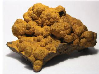
Iron is extracted from rocks such as **limonite** (central PA). Iron was used to make steel.
