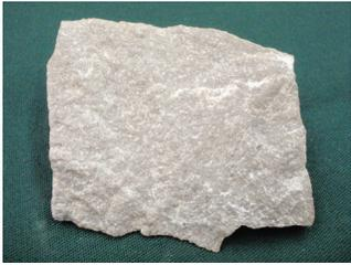
Limestone is used for building construction, for gravel, and for making concrete.
